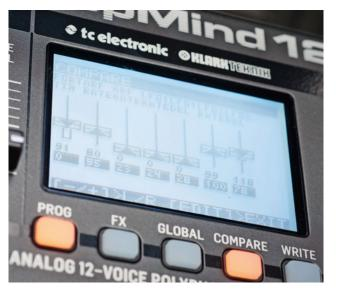
The quality of effects, and the scope for editing, is also high. For example, you can add a chorus followed by modulated hall reverb (inspired by the Lexicon 480L) that also feeds back into a pitchshifter and delay which is then routed into the reverb. Instant Eno/Lanois 'shimmer'.
